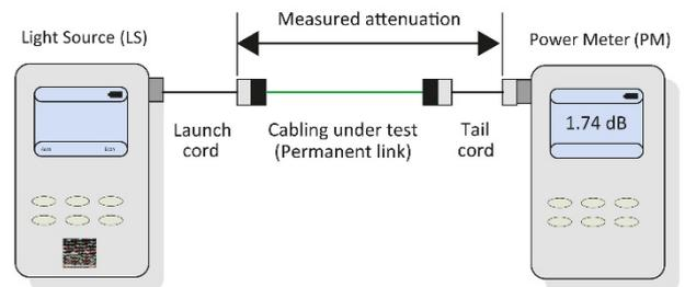
Figure 3: One-test-cord reference method, step 3
