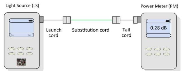
Figure 4: Three-test-cord reference method, step 2
