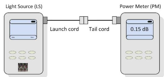
Figure 2: One-test-cord reference method, step 2
