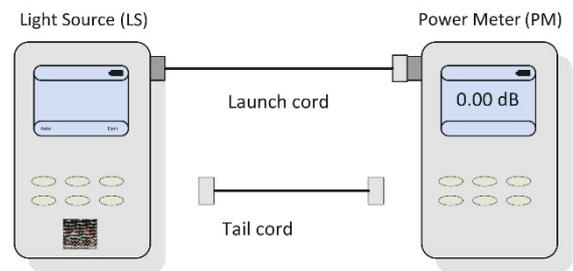
Figure 1: One-test-cord reference method and three-test-cord reference method, step 1
