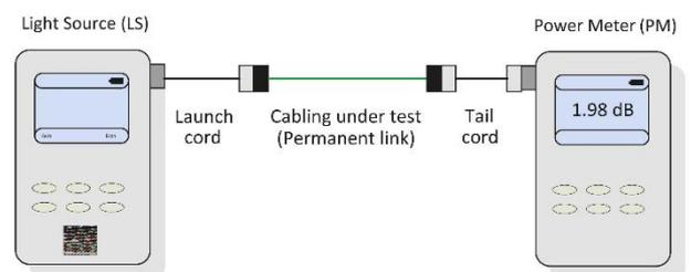
Figure 5: Three-test-cord reference method, step 3
