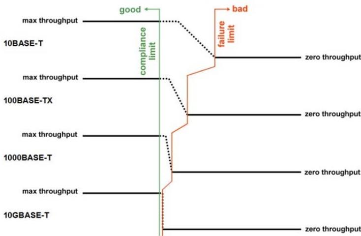
Figure 3: Operation of Ethernet BASE-T Systems with Non-compliant Cabling
