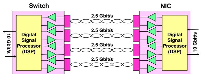
Figure 1: 4-pair full-duplex transmission used by 10GBASE-T
